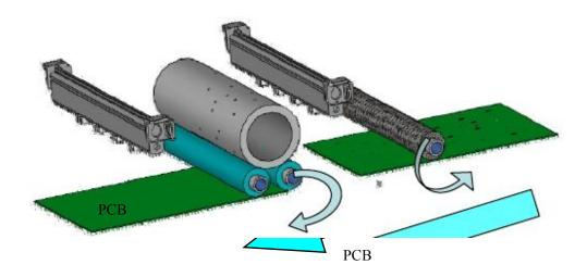
Single type wroking process :Cleaning PCB A side → PCB solder paste printing → Mounting → Reflow welding , PCB turnover machine → PCB B side cleaning → printing → Mounting → Reflow welding.
